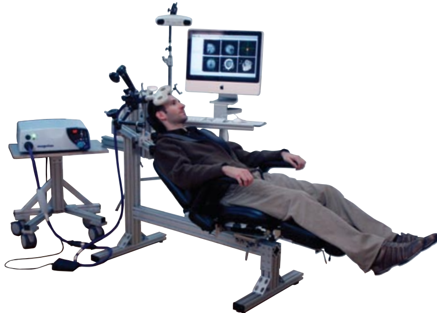
New TMS Chair with TMS coil holder arms
