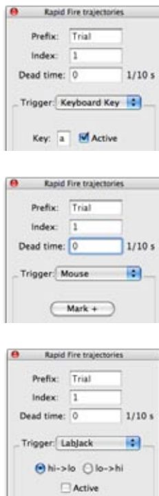
Rapid Fire Trigger windows (Marker tool and Trajectory tool), trigger via mouse click, keyboard key (typically for use with the X-Keys switch interface) or using the TTL input via the LabJack interface on certain Brainsight systems
