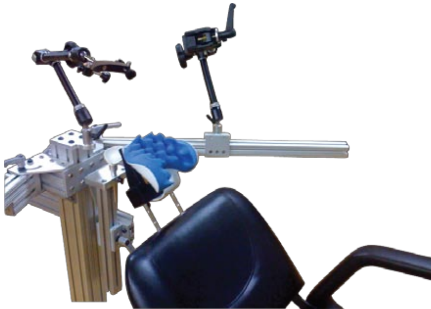
Top of stand with head rest and the arms in place
