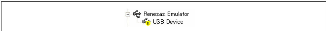
Figure 3.19 Display Indicating Failed Installation of a USB Driver
