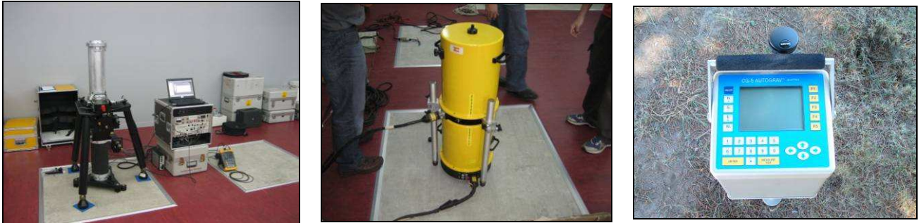
fig. 3 Gravimeters (FG5, A10 and Scintrex)
