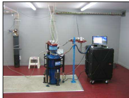
fig. 2 Observatory Superconducting Gravimeter
