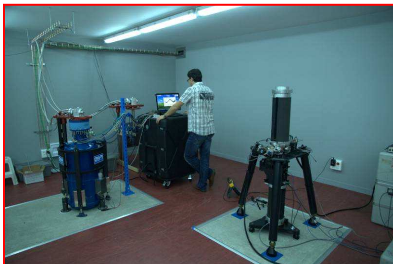
fig. 4 GWR-OSG and FG5 installed in Yebes
