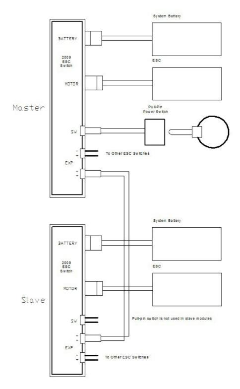
In the master-slave configuration, the switch can be connected to any module in the system. The expansion patch cables can be plugged into either of the two EXP connectors.
