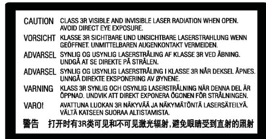
This label is located on the laser protective housing inside the product.
