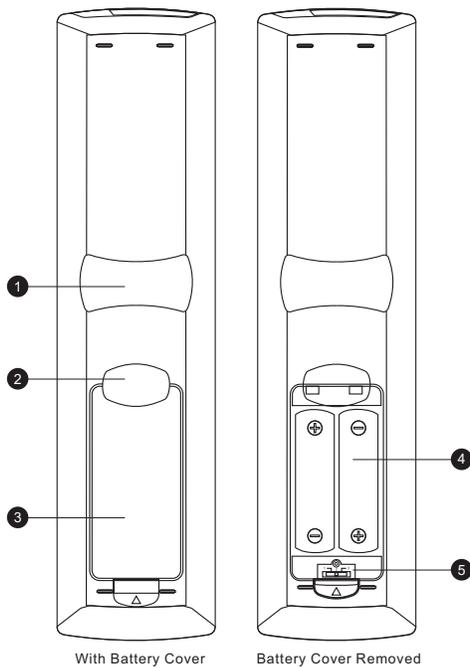
1. **Index Finger Notch 1:** When your index finger is placed at this notch while holding the remote control, your thumb is within easy reach of the navigation buttons (ARROW, ENTER, TOP MENU and POP-UP MENU).
