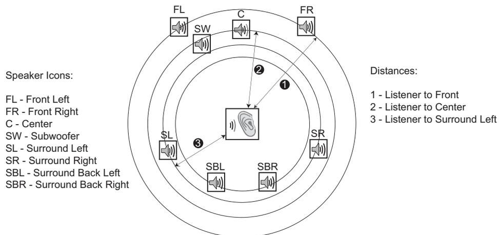
In the above diagram, measure the distance (in feet) from the primary listening position to the Front Left or Front Right Speaker. Enter the distance of the Front Speakers (❶ in the above picture) into the "Speaker Configuration" menu.
