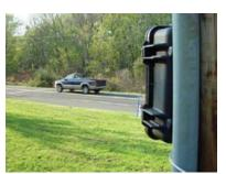
Again, note that it is the front of the Radar Recorder that you are aiming toward the road at a 45 degree angle.
