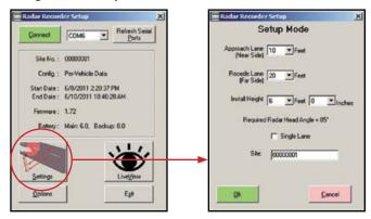
There are three lane configurations that are available for data collection: Normal Bidirectional mode, Reverse Bidirectional mode and Single Lane mode.
