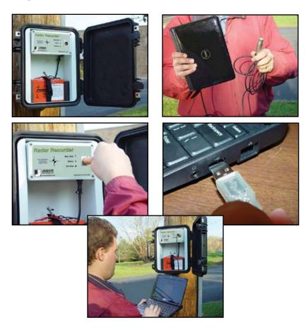
**NOTE:** The cable that connects the Radar Recorder to your laptop makes use of a USB serial adapter. This adapter requires that a USB driver be installed for it to work correctly. If you received your laptop directly from JAMAR, the driver has already been installed, so you do not need to worry about this.
