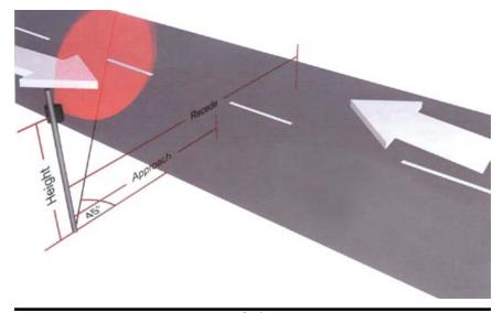
The distance from the Radar Recorder to the middle of the Approach Lane (near side) and the middle of the Recede Lane (far side), should be entered here, as well as the installed height of the Radar Recorder. Note that the lane distances should be measured directly from the pole to the road, as shown in the graphic.
