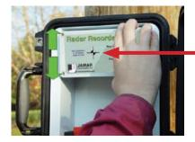
IMPORTANT: Note that the area of the Radar Recorder that you are aiming toward the road are the crosshairs printed on the face of the Radar head, as shown in the picture here.
