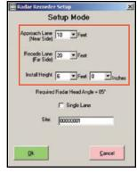
The Radar Head angle is set by rotating the Radar Head in the cabinet, which is discussed on page 3-6.
