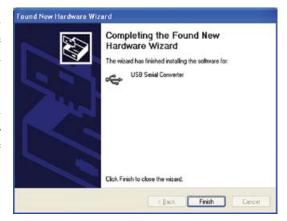
Once you click Finish, the Windows 'Found New Hardware' message will pop up again, referencing a USB Serial Port, and the *Found New Hardware Wizard* will reappear. Don't be alarmed, this is what's supposed to happen. There is a second driver that needs to be installed to create a virtual comm port.
