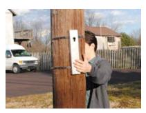
IMPORTANT: Note that the area of the Radar Recorder that you are aiming toward the road are the crosshairs printed on the face of the Radar head, as shown in the picture here.
