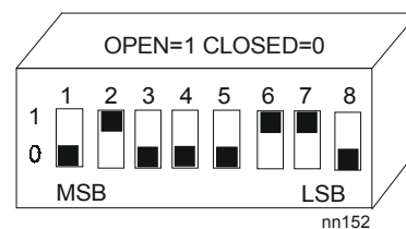
Figure 4: Switches with Fire OWS Node Number of 152
