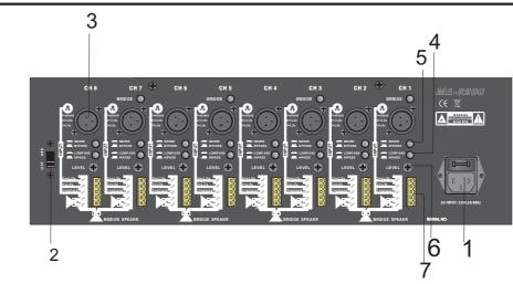
1. Mains jack for power supplu for connection to 230V~/50Hz
