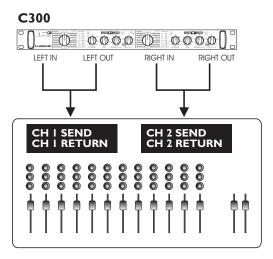
In this example the C300 is used in Dual Mono mode as two 100% independent mono engines on two separate channels. The two engines have no influence on each other.
