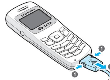
**Note:** Do not remove the battery from the phone without unplugging the adapter while it is charging. Otherwise, the phone may be damaged.
