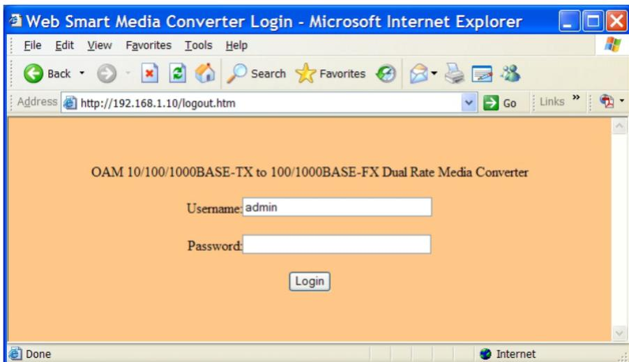
The default IP Address for the OAM Managed Media Converter is 192.168.1.10. Enter the factory default Username (admin). Enter the factory default Password (no password). Then click on the “Login” button to log on to the OAM Managed Media Converter.
