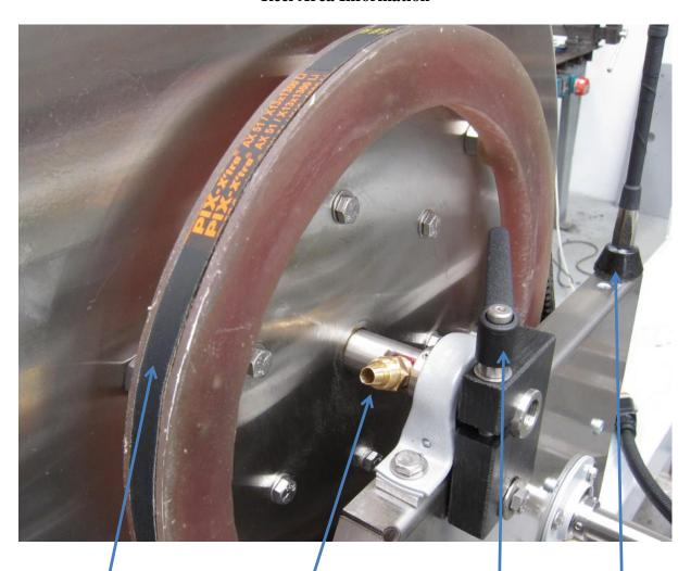
Reel drive belt. Belt type is an Automotive AX 51 Reel shaft compression fitting. The blue Supa Slip on the reel runs through the hole in the reel side and then is fitted to this fitting
