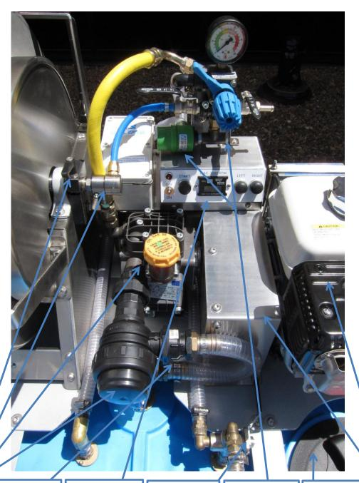
Reel break adjuster, reel swivel, PA 430 pump, pump oil glass and filter 2 way ball valve for tank shut off to filter when opening and cleaning of the filter Main control panel, tachometer, and remote engine start 3 way ball valve for changing from normal operation bypass back to tank to Pressure safety valve and pressure controller Tank lid area for filling tank with chemical and water Main drive guard and Honda motor
