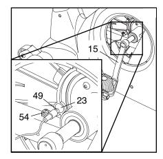
to or away from the Magnet. Then, retighten the Screw. Turn the Left Crank Arm for a moment. Repeat until the console displays correct feedback. When the Reed Switch is correctly adjusted, reattach the left Pedal Guard (8) and the left Side Shield Cover (14).
