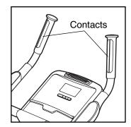
hold the handgrip pulse sensor with your palms resting against the metal contacts. **Avoid moving** your hands or gripping the contacts tightly.
