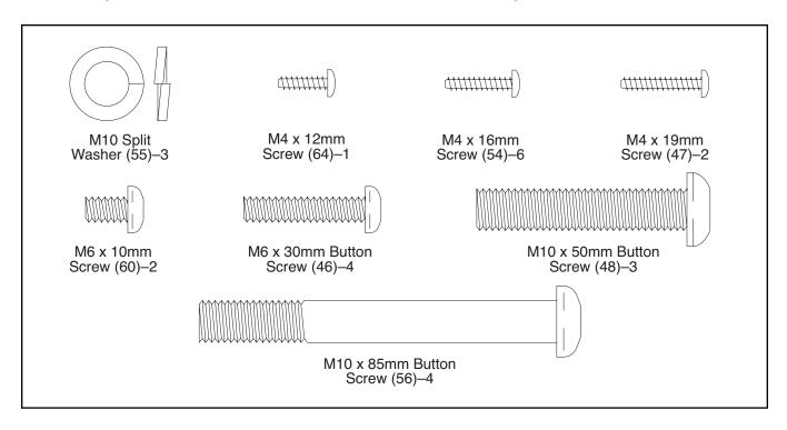
1. Attach the Front Stabilizer (2) to the Frame (1) with two M10 x 85mm Button Screws (56).
