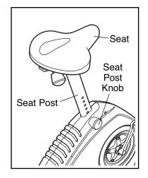
upward or downward to the desired position, and then release the knob. Move the seat post up or down slightly to make sure that the knob is engaged in one of the adjustment holes in the seat post. Then, turn the knob clockwise to tighten it.
