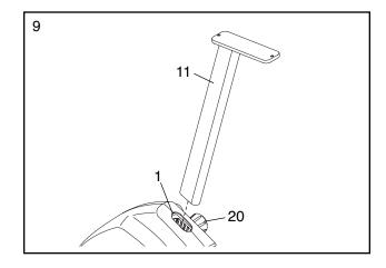
Attach an M6 x 10mm Screw (60) to the Seat Post (11). Next, slide the Seat Carriage (19) onto the Seat Post. Then, adjust the Seat Carriage to the desired position and tighten the Seat Knob (31) into the Seat Carriage.
