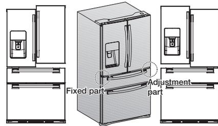
The left door is fixed. To make minor door adjustments, adjust only the right door.
