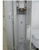
**2.** Connect the CO<sub>2</sub> cylinder to the regulator. Turn the CO<sub>2</sub> cylinder clockwise to install it.
