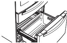
2. Remove the freeze room guard ( 1 ) by lifting the guard up.
