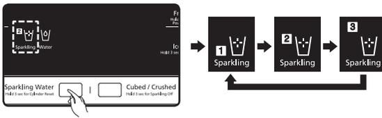
The Carbonation Level is set to Level 2 at the factory. If the sparkling water tastes too strong or too weak, change the carbonation level. Level 1 provides a milder carbonation, Level 3 a stronger carbonation.
