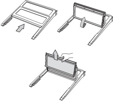
**CAUTION** After sliding the foldable shelf in and folding it, the Shelf Front can be removed for your convenience. If you use the self without removing, be careful of its possible separation.
