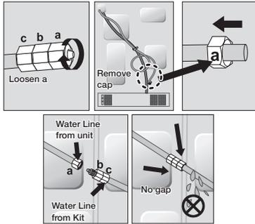
**CAUTION** ⚠ Before being used, the leakage in these places should be examined.
