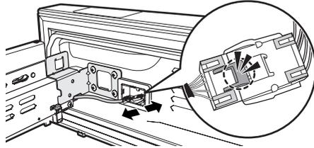
**CAUTION** When reassembling it, be sure to connect the wire harness. If it is not connected, the Flex Room does not work.
