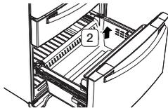
4. Press the fixing hook of the rail system.
