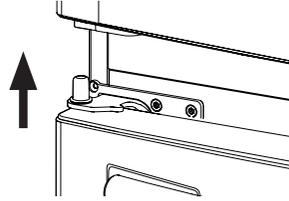
5. Remove the screw (8) attached to the lower left and right door hinges with a philips screwdriver (+). Remove the 2 hex head bolts (9) attached to the lower left and right door hinges with an allen wrench (5 mm). Remove the lower left and right door hinges (10).
