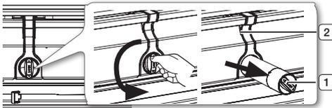
2. Pull the water filter ( 1 ) from the case filter ( 2 ).
