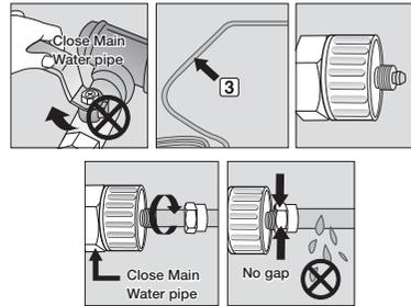
4. After connecting the water supply to the water filter, turn your main water supply back on and dispense about 3L to clear and prime the water filter.
