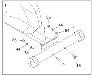
While another person lifts the front of the Frame (1), attach the Front Stabilizer (6) with two M10 x 70mm Carriage Bolts (16), two M10 x 1,5mm Washers (54), and two M10 Nylon Locknuts (44). Next, press two Acorn Covers (35) onto the Nylon Locknuts.
