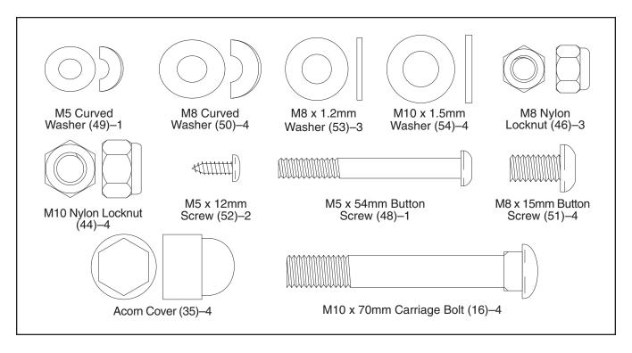
While another person lifts the rear of the Frame (1), attach the Rear Stabilizer (7) to the Frame with two M10 x 70mm Carriage Bolts (16), two M10 x 1,5mm Washers (54), and two M10 Nylon Locknuts (44). Next, press two Acorn Covers (35) onto the Nylon Locknuts.
