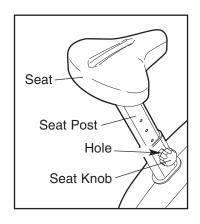
Next, slide the seat post upward or downward to the desired position, and align one of the adjustment holes in the seat post with the indicated hole in the frame. Then, insert the knob into the frame and the seat post, and turn the knob clockwise until it is tight. Make sure that the knob is inserted into one of the adjustment holes in the seat post.
