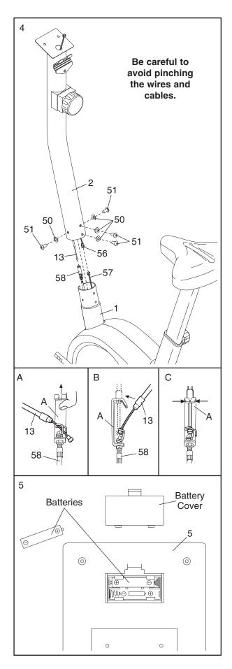
6. Have another person hold the Console (5) near the Upright (2). Connect the console wire to the Upper Wire Harness (56). Then, connect the console pulse wires to the Upper Pulse Wires (66) as shown.
