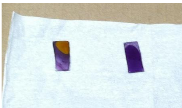
Figure 4-22. P3HT films dropcoated from chloroform solution as the solvent evaporates. Left: 0% Hg3, Right: 50% Hg3
