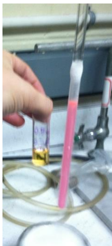
Figure 4-15. Color change of MEH-PPV in methyl THF upon freezing to liquid nitrogen temperatures. Vial, right: MEH-PPV in methyl THF at room temperature. Tube, left: MEH-PPV in frozen methyl THF.
