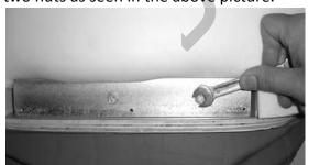
7. User the wrench to turn right nut 360 degrees in clockwise. The nuts will cause the cable to break over too much tension.
