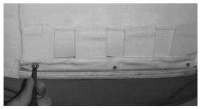
3. Remove all three screws by applying the proper screw driver.
