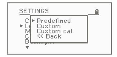
The **Predefined** option allows to select one of the predefined slider lengths **(1.0m, 1.5m, 2.0m or 2.5m)**.
