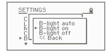
In **Backlight Auto** mode the the LCD display will be dimmed automatically after a certain period of time if the device is not operated. Use this option to maximize battery life and avoid unnecessary light artifacts on your long exposure timelapse shots.
