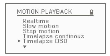
The drive-shoot-drive timelapse playback menu has similar features to standard timelapse. However, the direction feature is not present here as the playback because always performed from the home position along the recorded path.
