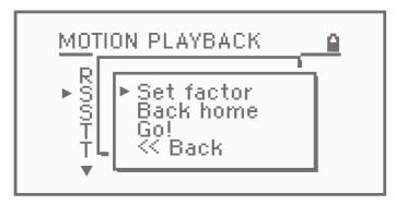
**Set Factor** option allows you to set the desired stretch factor of the recording. The playback time will be multiplied by an integer of your choice.
