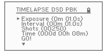
You may set the Exposure time, the Interval time, and the total Shots. Adjusting the Time parameter will re-calculate the total Shots automatically.
