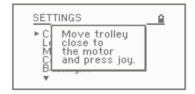
If the trolley hits the end of the track and you hear the internal controller warning sound, press the internal controller reset button (servo only) and confirm the calibration with the joystick.
