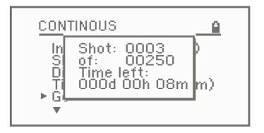
If you move the joystick up or down during the progress of the timelapse sequence, the additional parameters are displayed:
