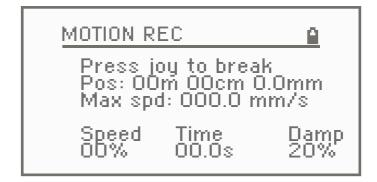
After selecting the Motion recording mode the current position of the trolley is registered as home position. All playback will be started from that position.
