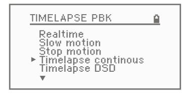
The continuous timelapse playback menu has similar features to standard timelapse. However, the direction feature is not present here because the playback is always performed starting at the home position along the recorded path.
