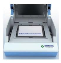
Note: Gel Window is used as the spacer between anode pad and cathode pad to prevent short circuit. The edges of the pre-run gel may also be covered by Gel Window and will probably be stained to deep blue after running an electric staining program.
