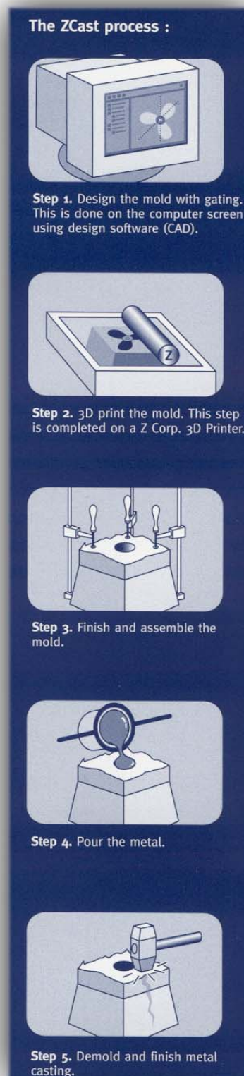
Figure 5: Steps involved in using ZCast powder
