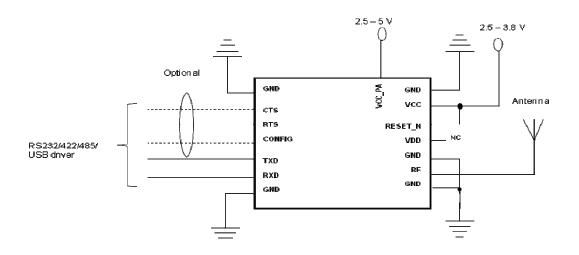
Note that the VCC\_PA pin is only connected to 5V for the RC1700HP to achieve +27 dBm. If VCC\_PA is connected to VCC the max output power for the RC1700HP is +24 dBm. For RC1700 and RC1700MP the VCC\_PA should be left open (not connected).
