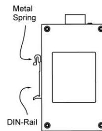
Reverse Steps 1 and 2 above to remove the VPort 451 from the DIN-Rail.
