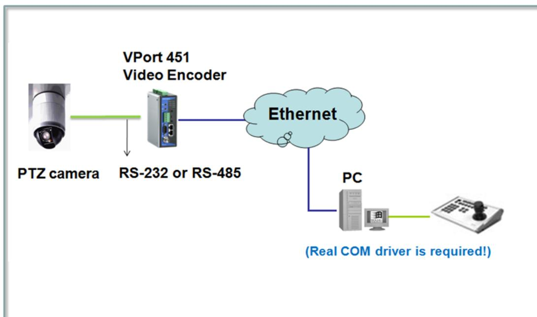
**NOTE** The PTZ control protocol is not standardized. To use a particular PTZ control protocol, the video server must support the driver for that protocol. Currently, the VPort 451 supports PTZ control protocol drivers for:
