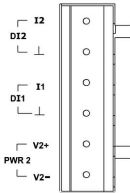
The VPort 451 has two sets of digital inputs, DI1 and DI2. Each DI consists of two contacts of the 6-pin terminal block connector on the VPort’s top panel. Top and front views of one of the terminal block connectors are shown here.
