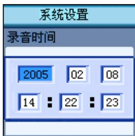
3. Short press the VOL + key to set up the year (VOL - for opposite direction), the display for the year begins to flash.
