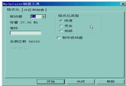
3) In the formatting tool which is shown up first, select "Partition and Encryption", select a suitable capacity for the encrypted partition, check select the option for user name and password, in the "New user name" field, input the user name, in the "New password" field, input the password, in the "Confirm new password" field, input the same password, click "Start" to start the partition process.
