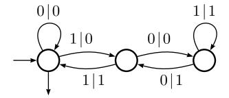
The transducer computing the quotient by 3 of a binary number.
