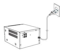
Connect the power cable to the wall socket.
