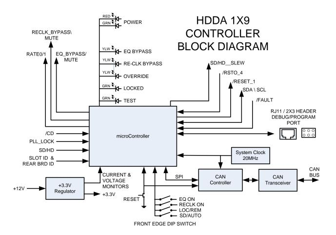
The PIC32 microcontroller, PIC32MX340F256H, was chosen based on cost and familiarity of the engineering staff with this device. In order to be able to communicate over the CAN bus in the openGear frame a CAN Controller IC, MCP2515 in conjunction with a CAN bus transceiver, SN65HVD233D, is used. The CAN Controller is controlled by the PIC32 using the SPI2 port of the PIC.
