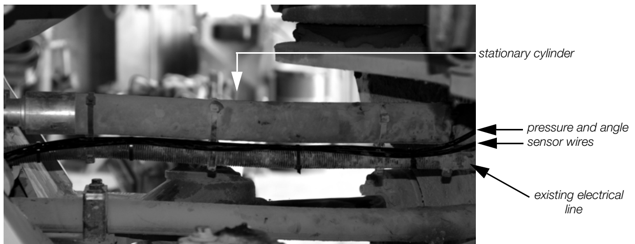
Figure 1-17. Wires Routed Along Existing Electrical Line.
