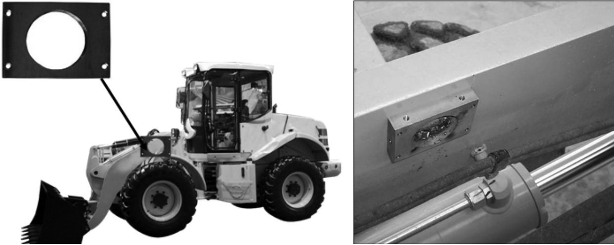
Figure 1-13. Weld The Angle Sensor Mounting Plate Onto The Support Arm
