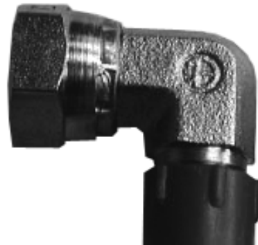
Figure 1-8. 1/4" NPT male to 1/4" BSPP Female Swivel 90-Degree Fitting
