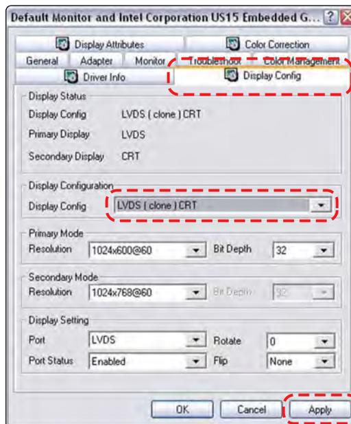
Figure 14-4 Sample Display Config tab
