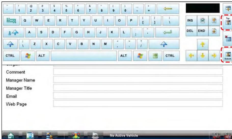
Figure 13-5 Virtual keyboard Top and Bottom buttons
