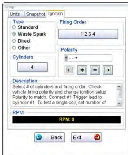
Figure 8-30 Sample Setup Ignition dialog box
