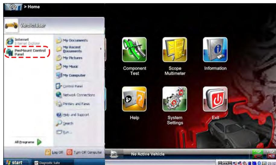
Figure 14-1 Launching the calibration program
