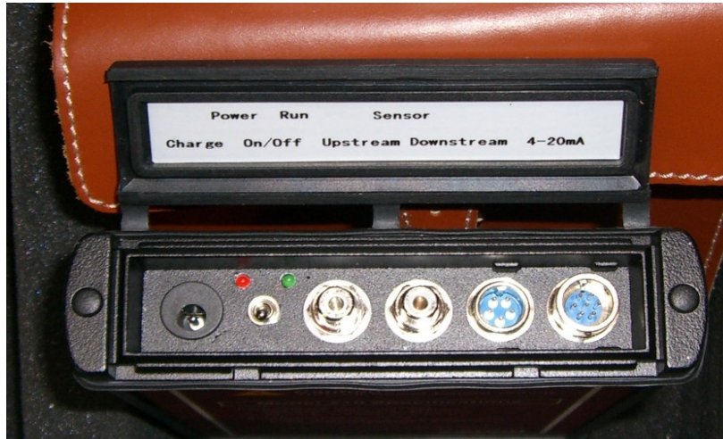
Figure 2-1 INNOVA SONIC PORTABLE Panel and Connection Diagram
