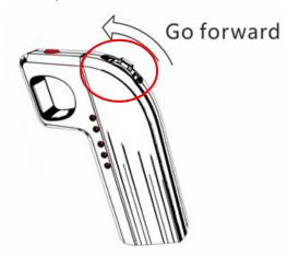
**Fifth:** when you meet red traffic light or there is another thing need to stop skateboard, there are two ways. One is operation as above forth step(loose the slide button, the speed will reduce to zero and stop), the other way is sliding the button to backward direction to brake, the skateboard will stop;
