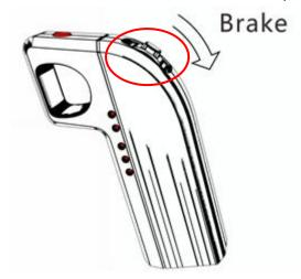
**Note:** the only difference of these two stopping way is brake need less time ,but loose slide button to middle place need speed reduce to "zero":
