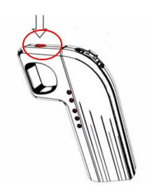
**Third:** the indicator of "low speed" will light green, it means the skateboard is under "slow speed" mode; "low speed" model is the system default, every start of remote controller is the same;
