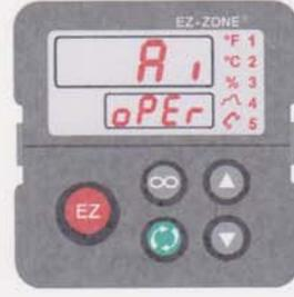
**Operations Page from Home Page:** Press both the Up  $\blacktriangle$  and Down  $\blacktriangledown$  keys for three seconds.
