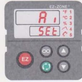
**Setup Page from Home Page:** Press both the Up  $\blacktriangle$  and Down  $\blacktriangledown$  keys for six seconds.
