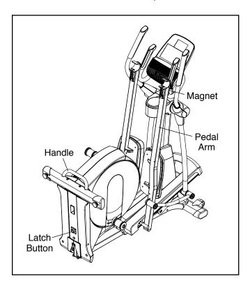
To use the elliptical, first hold the handle, press the latch button, and lower the frame.
