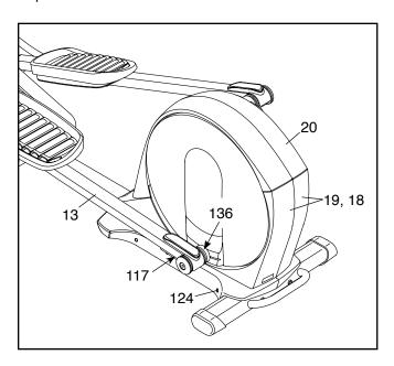
Next, lift the Latch (117) on the underside of the Left Pedal Arm (13), and then lift the Left Pedal Arm off the left Sleeve (136). See EXPLODED DRAWING B on page 37. Remove the M4 x 16mm Screws (93) and the M4 x 42mm Screws (124) from the Right and Left Shields (18, 19). **Make sure to note which size Screws come from which holes.** Then, carefully remove the Left Shield.
