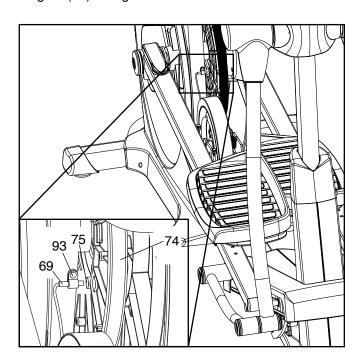
Next, loosen, but do not remove, the indicated M4 x 16mm Screw (93). Slide the Reed Switch (69) slightly toward or away from the Magnet (75). Then, retighten the M4 x 16mm Screw.
