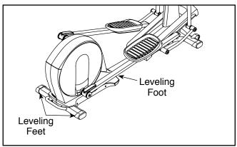
If the frame of the elliptical flexes during use, turn the center leveling foot until the flexing motion is eliminated.
