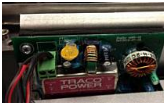
Figure 2 - 1. 24 V DC Power Supply Terminals.
