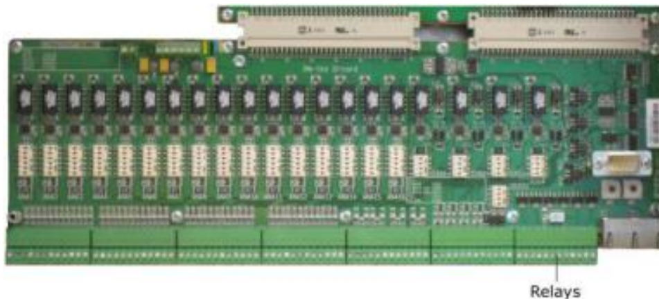
Figure 3 - 5. IMx-B I/O Board, Relays.
