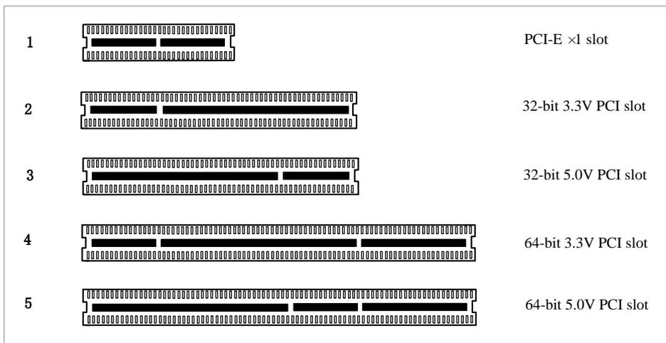
Figure 2 PCI-E and PCI slots
