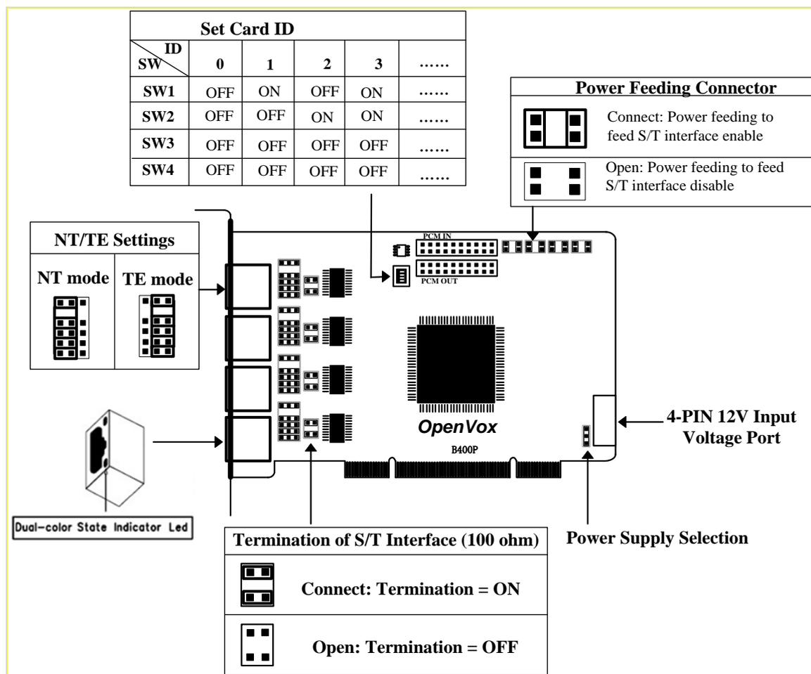
Figure 3 Jumper setting
