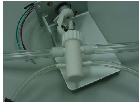
Example of pump with rinse ports at rear of pump (note: hose clamps have been removed for photo clarity).
