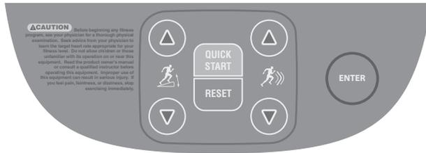
**CROSSRAMP**—Press and hold the CROSSRAMP arrow keys to increase or decrease the ramp incline from 1 to 8.
