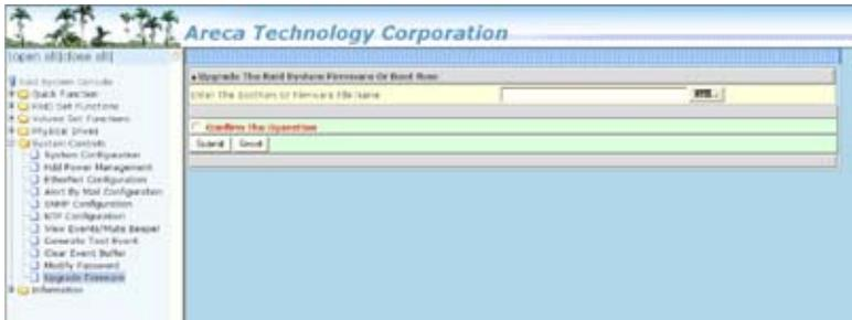
1. To upgrade the SAS RAID controller firmware, move the mouse cursor to "Upgrade Firmware" link. The "Upgrade The Raid System Firmware or Boot Rom" screen appears.
