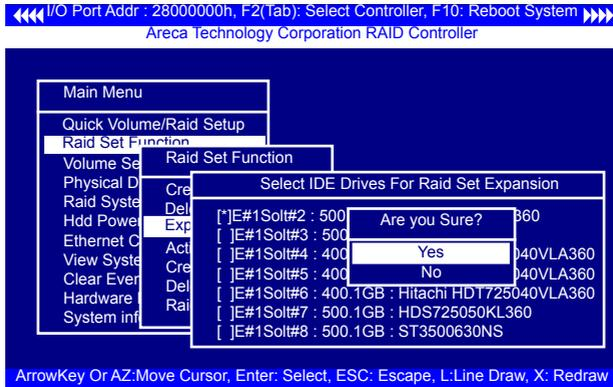
Instead of deleting a RAID set and recreating it with additional disk drives, the "Expand RAID Set" function allows the users to add disk drives to the RAID set that have already been created. To expand a RAID set:
