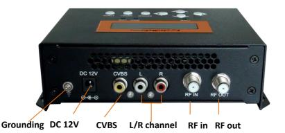
Grounding: to connect the earth cable
