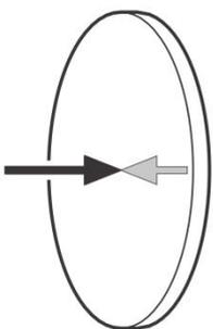
When an object is held up to the coated side there is no space between the object and its reflection. The back edge of the gobo cannot be seen when looking through the coated side.
