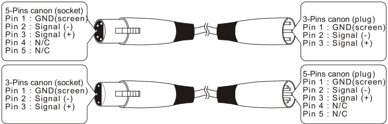
3. Link the units as shown in (figure 5), Connect a DMX signal cable from the first unit's DMX "out" socket to the second unit's "in" socket. Repeat this process to link the second, third, and fourth units.
