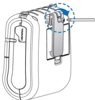
(2) Tighten the screw with driver as shown.
