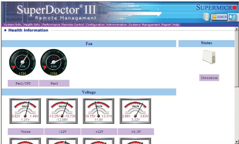
Figure 2-8. SuperDoctor III Interface Display Screen (Health Information)
