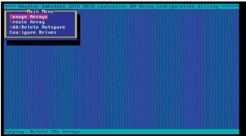
Figure 2-5.Adaptec RAID Utility Program Screen
