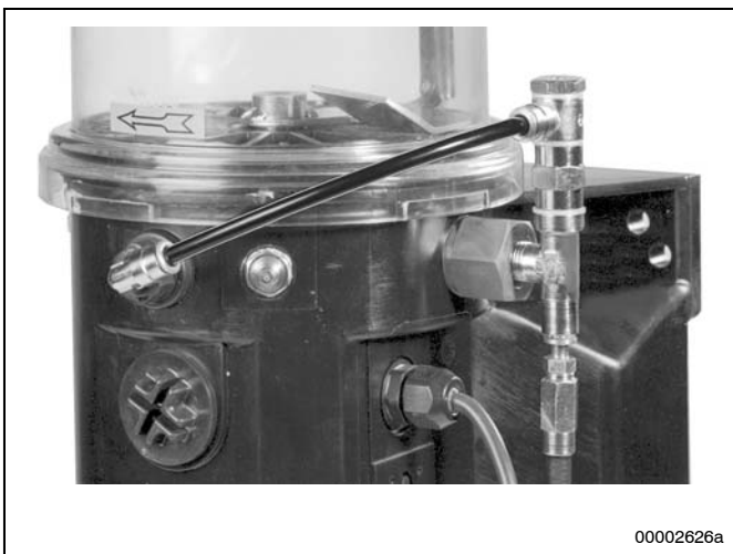
Fig. 17 Pressure relief valve with grease return
