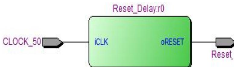
Fig.7. RTL View of Reset Block
