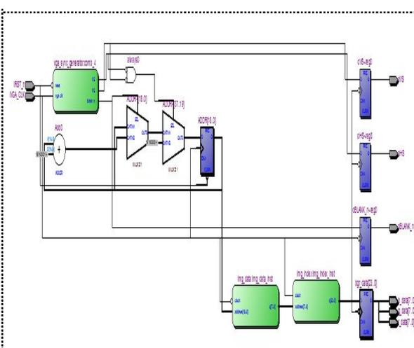
Fig.12. RTL View of Internal VGA Controller
