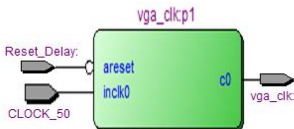
Fig.3. RTL View of Clock Generator Block
