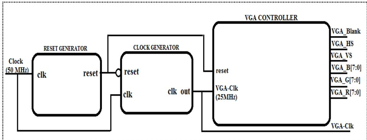
Fig1. Proposed Block Diagram
