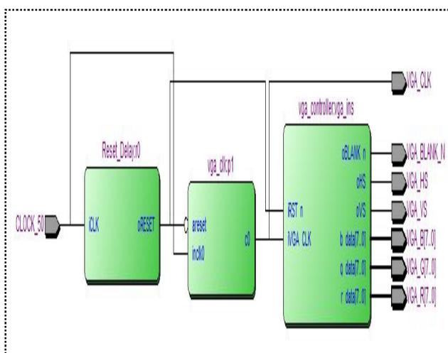
Fig.11.RTL View of VGA Controller
