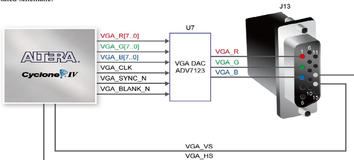
Fig 8. Connections between FPGA and VGA
