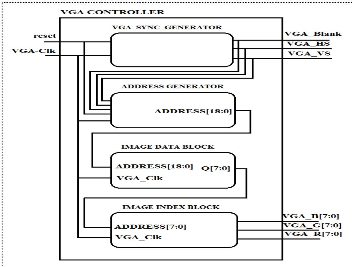
Fig.2. Internal Block Diagram Of VGA Controller.
