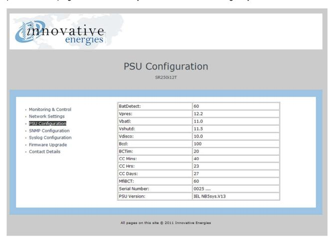
The basic model number of the power supply unit is shown below the 'PSU Configuration' heading. In the screenshot above you can see that it is displayed as SR250i12T.
