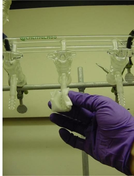
Step 38: Clean the manifold stems to which each rubber tube will be attached.
