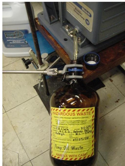
Step 32: Drain the old vacuum pump oil into an appropriately-labeled and properly-secured oil waste container.
