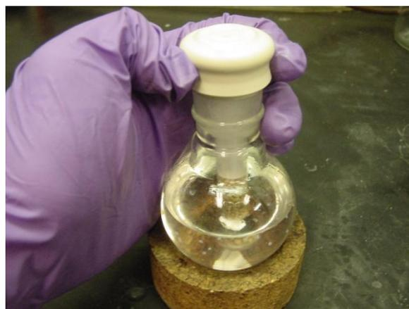
Step 12: Insert the molecular sieve holding device into the reaction flask and secure the septum.
