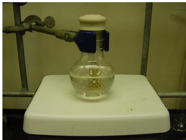
4A molecular sieves are useful for removing equilibrated  $\text{H}_2\text{O}$ ,  $\text{CH}_3\text{OH}$ , or  $\text{CH}_3\text{CH}_2\text{OH}$  reaction byproducts. The improvised molecular sieve holding device is useful for keeping the sieves from contacting the magnetic stir bar.
