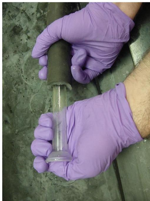
Step 28: Insert half the length of the glass stem into the rubber tubing.
