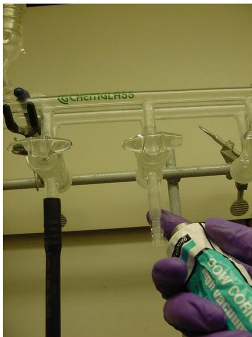
Step 39: Apply a thin coat of high vacuum silicon grease to each stem before attaching each tube.
