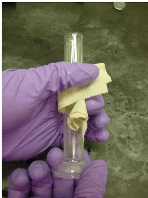
Step 25: Use a hexane-soaked paper towel to clean the glass stem of the manifold / tube connecter.
