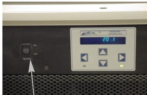
Open the cabinet. Flip the switch to the off position and leave it there to turn the heater off manually.
