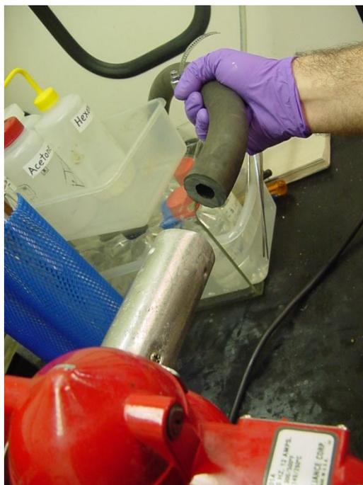
Step 27: Soften the grease applied to the inside of the rubber tubing by heating briefly with a heat gun. This will make it much easier to insert the glass stem.
