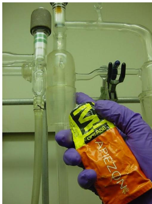
Step 20: Apiezon grease is especially recommended for the manifold / trap connection.
