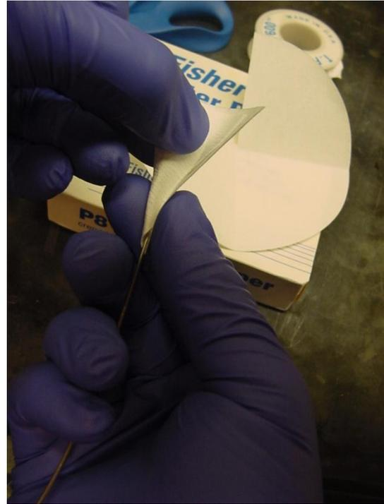
Step 4: Fold the right side of the quarter cut, as well as the overlap from the left side fold, back across the top of the needle hilt.
