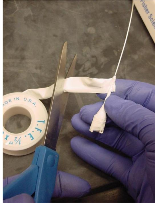
Step 10: Cut the tape from the roll, sparing several inches with which to tie the tape to the needle.
