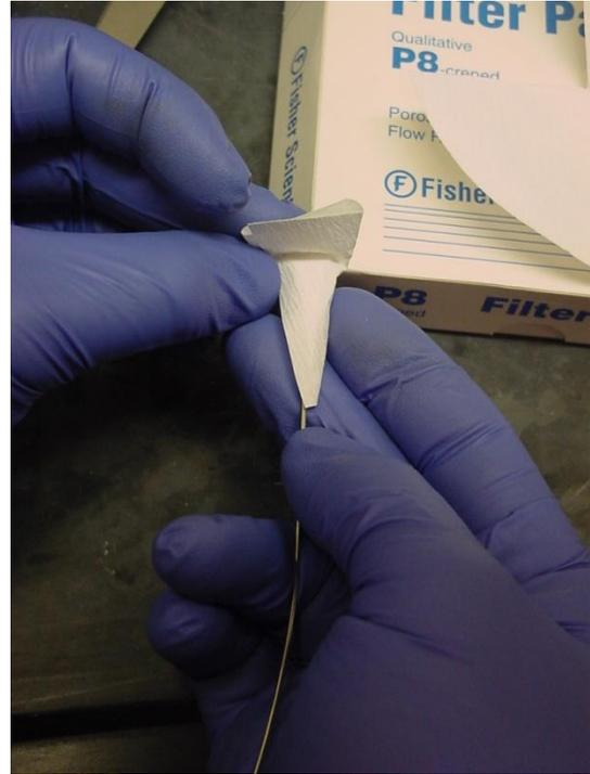
Step 6: Fold the top of the cone down and over the needle hilt until it is flush with the opposite side.
