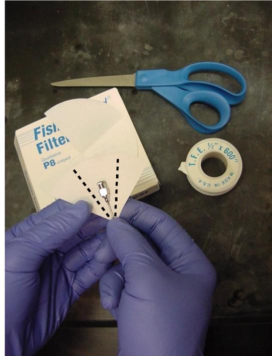
Step 2: Position the hilt of a 12 inch, 18-gauge needle at the center of the quarter cut as shown. Folds to be made in Steps 3 and 4 are outlined by the dashed lines.
