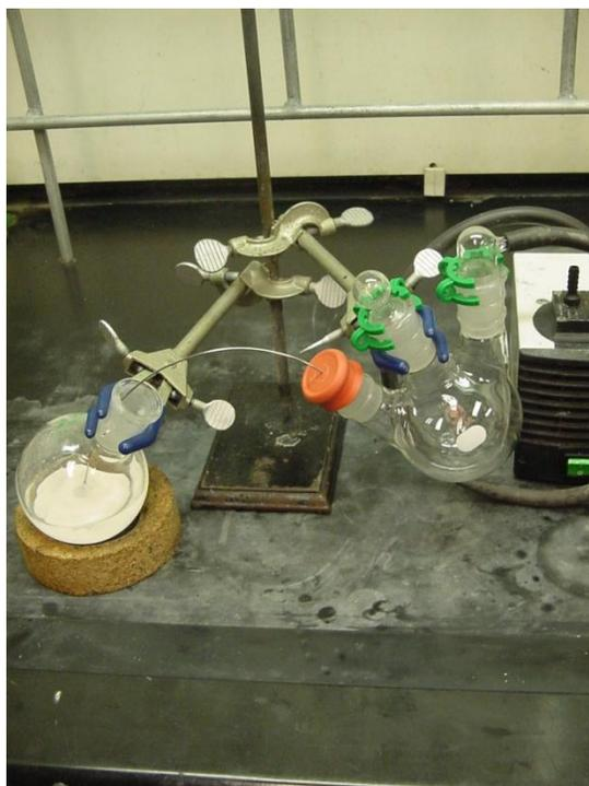
Step 15: Puncher the rubber septum with the sharp end of the needle.
