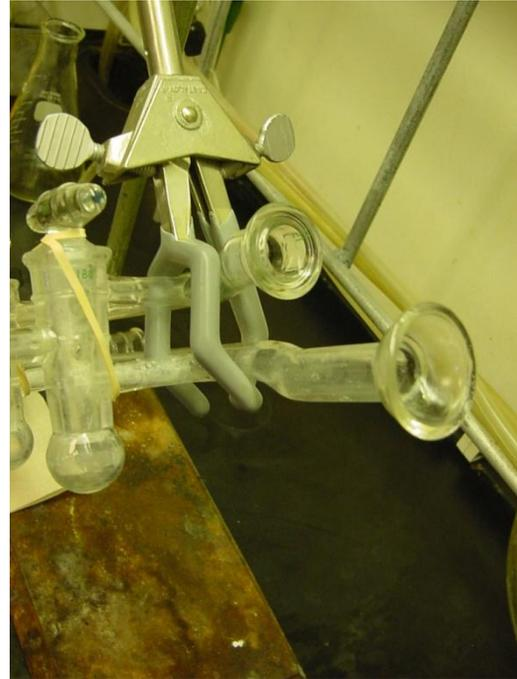
Step 2: Tighten a three-prong clamp on the manifold at the first set of joints from the open end of the vacuum line such that the two-pronged side of the clamp sandwiches the joints leading to the stopcock as illustrated.
