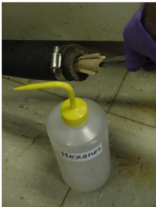
Step 31: Use a hexane-soaked paper towel on a long pair of needle-nose tweezers to remove old grease deposits from the tubing.
