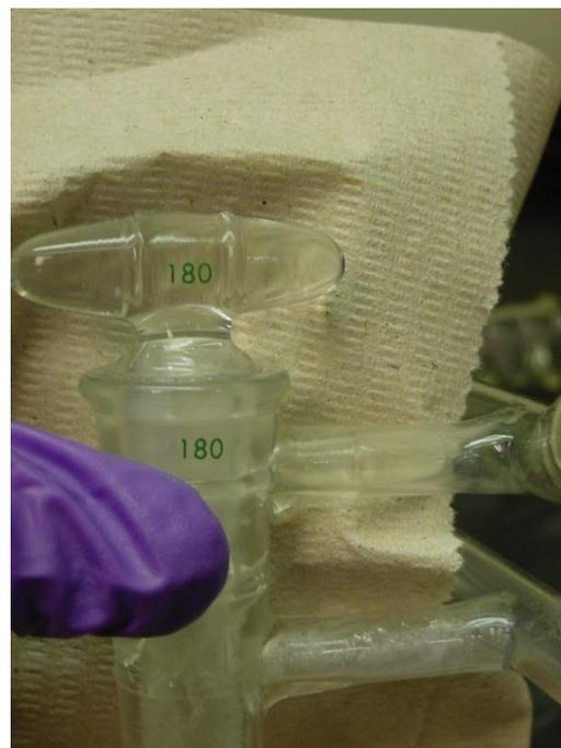
Step 16: Return each stopcock to its properly-numbered joint. Double check that the joint number matches the stopcock number, as each custom fit maximizes the vacuum capability of the system.
