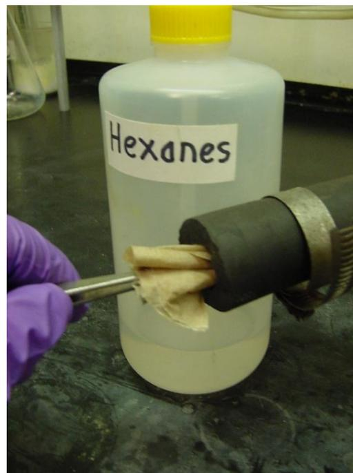
Step 22: After trimming off the damaged portion of the tubing, clean the end section of old grease deposits by use a long pair of needle-nose tweezers to insert and withdraw a hexane-soaked paper towel with a twisting motion.
