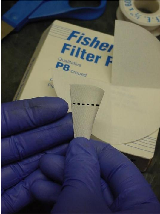
Step 5: At this point, the folds should amount to a cone over the needle hilt. The next fold to be made is outlined by the dashed line.
