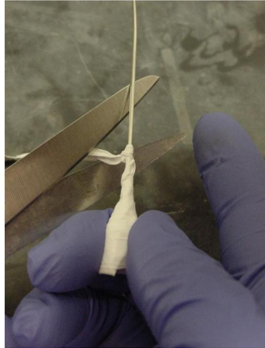
Step 12: Pull the overhand knot tight and cut off the extraneous tape at the loose end.
