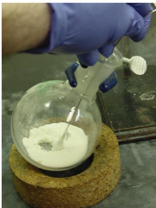
Step 17: Reposition the filter paper-covered needle as needed to suck the last standing remnants of supernatant from the bottom of the flask.
