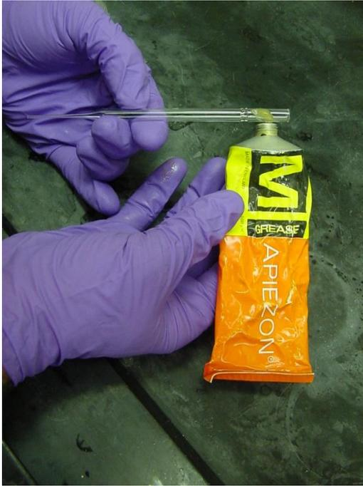
Step 23: Smear Apiezon grease on the thick end of a glass pipet.
