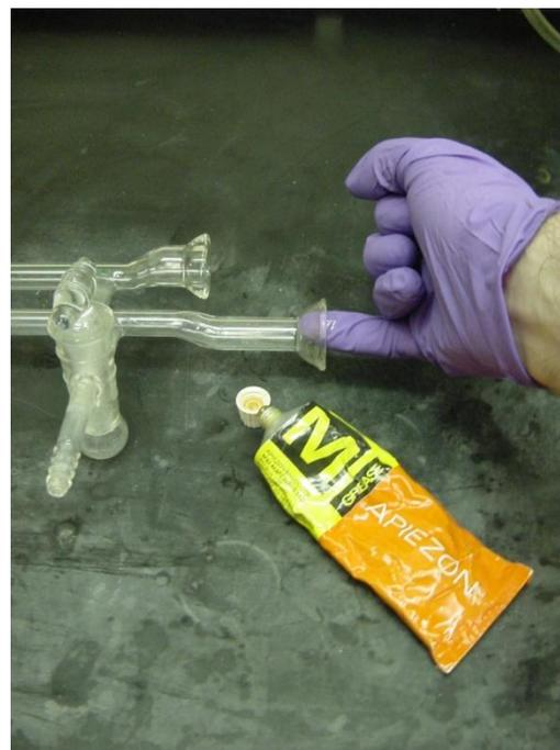
Step 18: Apply a fresh coat of hydrocarbon grease to each joint after removing the old grease. Apiezon grease is recommended for stationary connections, such as ball-and-socket joints.
