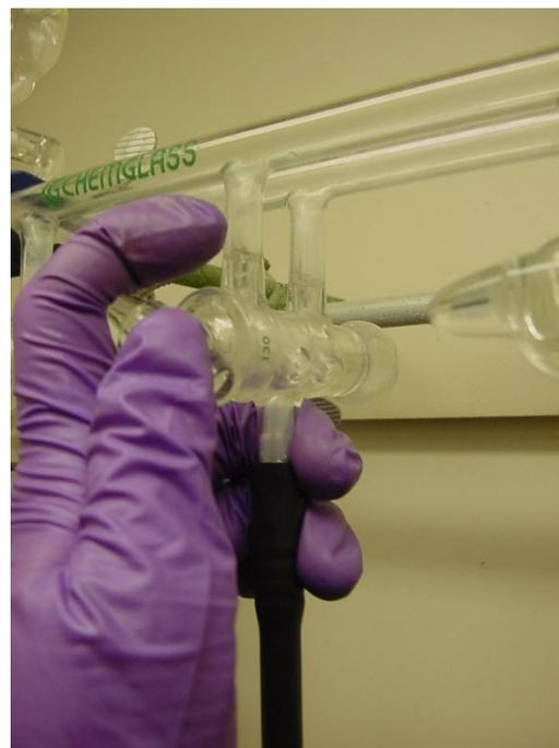
Step 40: Turn the vacuum pump on. Twist and press each stopcock to uniformly distribute the silicon grease and tighten the seal. Each stopcock should rotate smoothly. If not, remove the stopcock and apply more grease.
