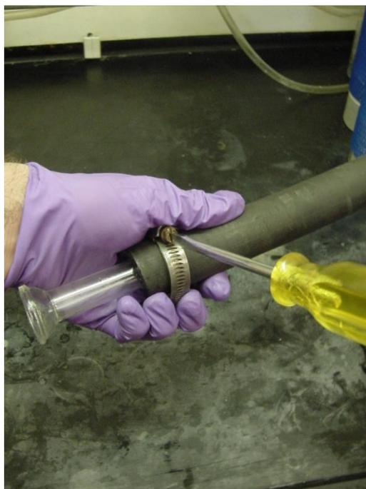
Step 29: Secure the connection with a hose clamp.
