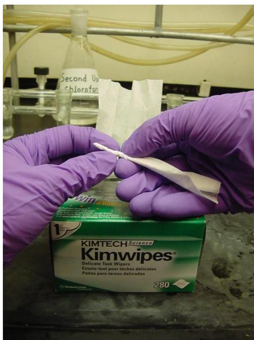
Step 9: Grease-clogged stopcock channels can be cleaned with a Kimwipe. Tear a Kimwipe in half widthwise, roll it, and twist one end of the roll into a tight point.
