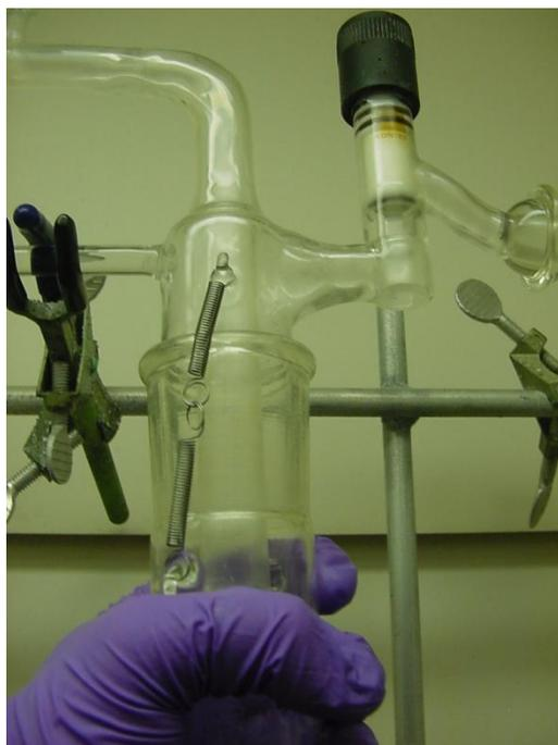
Step 41: Gently twist the cold traps back and forth under vacuum to ensure a proper seal. As with the stopcocks, apply more grease if the traps fail to rotate smoothly and easily.
