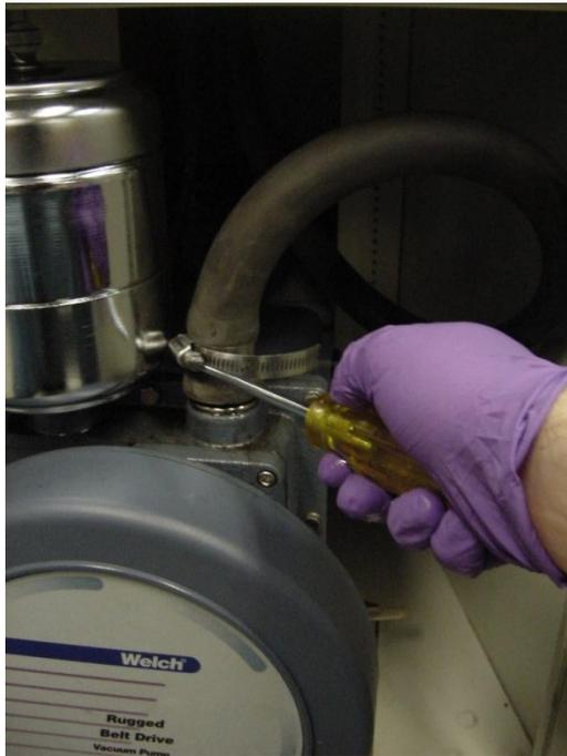
Step 35: Attach the tubing to the vacuum pump and secure the connection with the hose clamp as illustrated.
