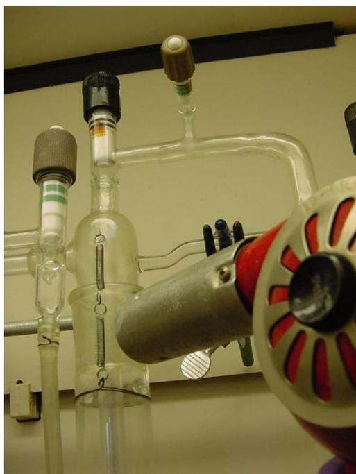
Step 19: Remove the cold traps and clean off the old grease from the contact surfaces.
