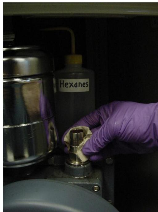
Step 30: Disconnect the rubber tubing from the vacuum pump and use a hexane-soaked paper towel to clean the vacuum pump, tube connector.
