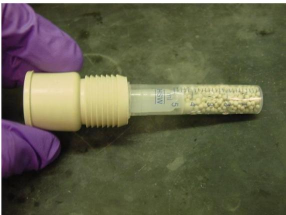
Step 11: Re-insert the plunger into syringe. The three puncher holes at the 5 mL mark will function as tabs to secure the plunger in the syringe.
