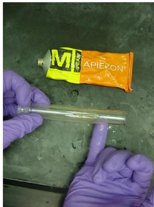
Step 26: Apply Apiezon grease to the half of the glass stem to be inserted in the rubber tubing.
