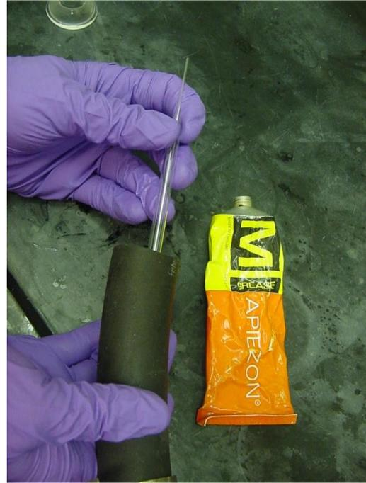
Step 24: Use the pipet to apply a fresh coat of grease several inches deep on inside of the rubber tubing.
