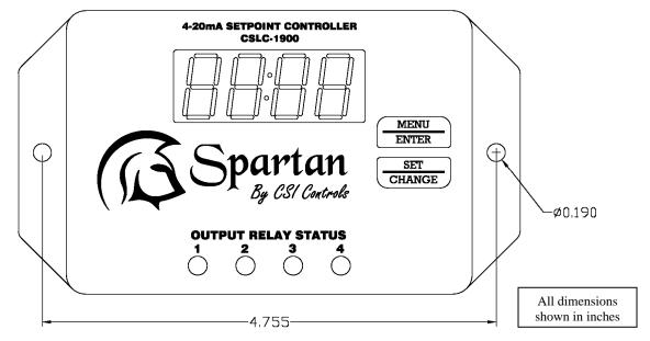
In the optional door-mount configuration, the Spartan is to be mounted behind a door or panel, with a rectangular cutout for front-side access to the front face of the controller.  $1^5/8$ " screws are suggested, using a  $1\frac{1}{4}$ " spacer as shown in the next figure. The door/panel cutout size and hole layout is also shown.
