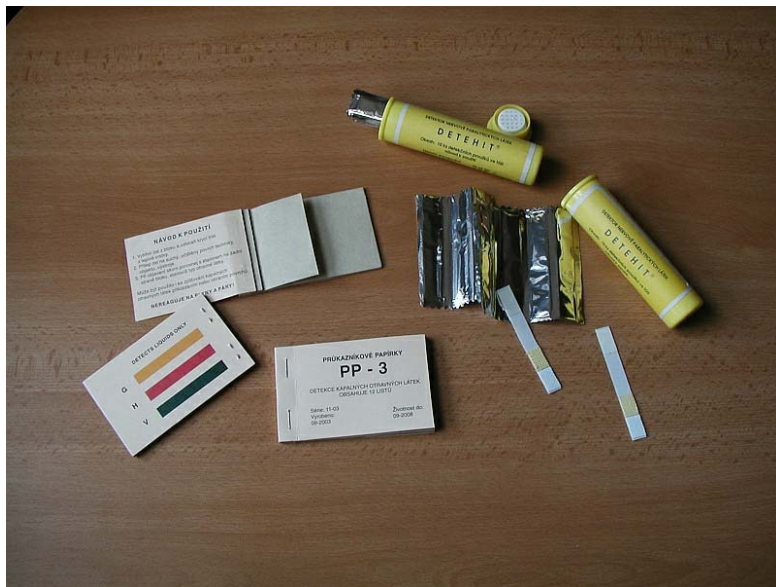
Pic. 2 Detection papers PP-3 and nerve-agents detector Detehit
