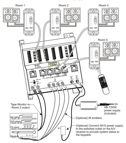
Most A/V receivers have a 'Tape Monitor' or 'Room 2' output that can be used to feed directly into the local input on the P-1014. This input is audio sensed so the keypad will mute when no signal is present.
