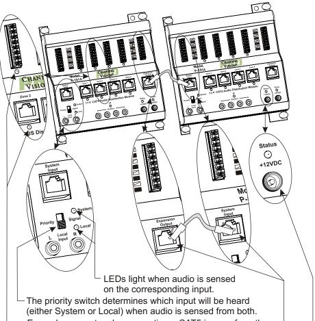
**Optional** Status power input senses when a connector is plug into it.—If the plug is connected and no power is present: The keypads will mute. If the plug is connected and power is present: The keypads will not mute. If nothing is plugged in: the system will still work normally.
