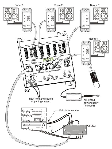
When using an AB-202 with the P-1014, the local source input can be used as a secondary input that overrides signals from the AB-202 whenever audio is present. This can be used as a whole-house paging input.
