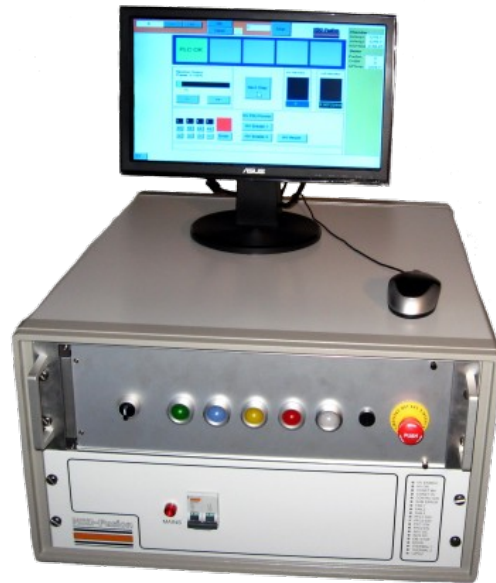
NSD Central Control Unit and 1.8 kW DC HV PSU enclosure. A typical industrial PC and its I/O modules plus power switching relays and 24 volt DC power supply can be accommodated in a 3U 19" sub-rack or similar enclosure.
