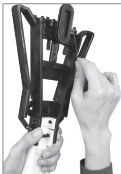
Grip the neck and wind the coil wire around the pickup. Use the hand holding the coil wire to straighten the wire while winding.
